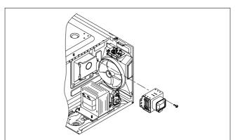
**NOTE**: Never install the magnetron without the metallic gasket plate which is packed with each magnetron to prevent microwave leakage. Whenever repair work is carried out on magnetron, check the microwave leakage. It shall not exceed 4mW/cm² for a fully assembled oven with door normally closed.
